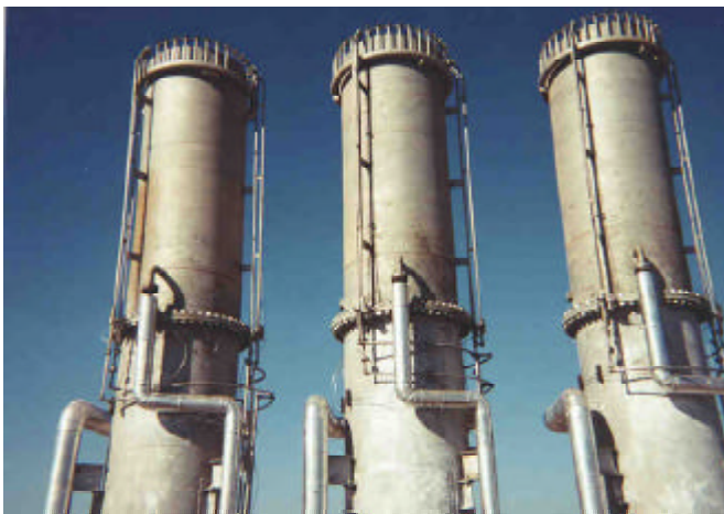
Three QFS Flares with Center Steam Sparger
