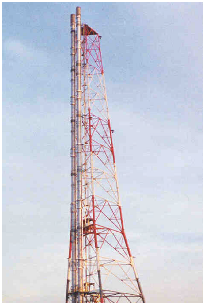
Two QFS-72 Flares with Demountable 492' Stacks
